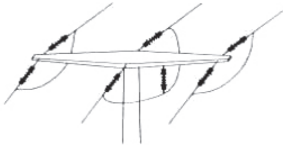
Insulated conductors minimum of 70 cm on each side of cross arm (taken from Haas et al. 2003)
