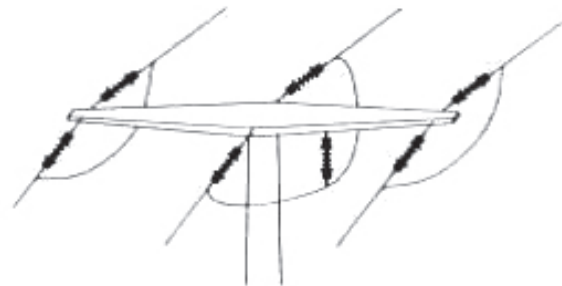
Insulated conductors minimum of 70 cm on each side of cross arm (taken from Haas et al. 2003)
